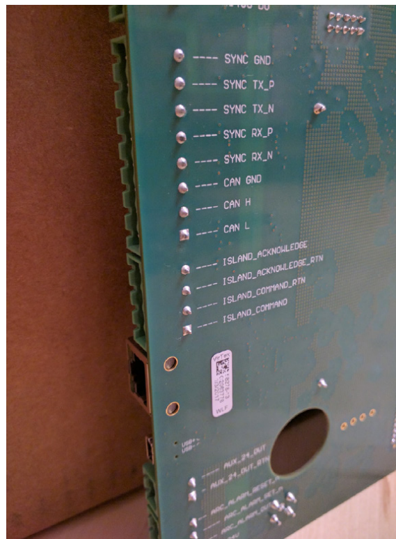
Figure 3. PCS control board connections including ISLAND_COMMAND & ISLAND_ACKNOWLEDGE
