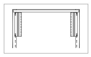
Fix the bracket with supplied mounting screws.
