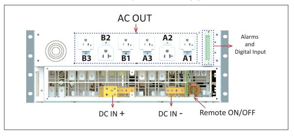
Note: Bravo ST 120 Vac has four different AC output connections. Refer to section 8.4, page 24, to identify the configuration which you received.
