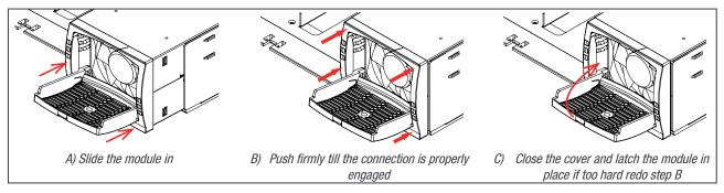
Once the module is inserted correctly and locked, it will restart automatically and begin to share the load. The sequence might take 10 to 40 seconds.
