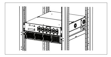
Fix the system in the rack with supplied mounting screws.
