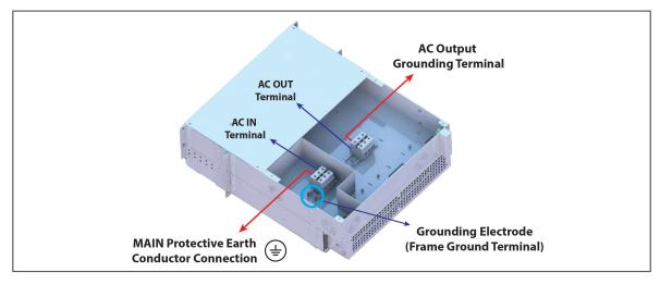
Ground has to be connected in accordance with local code.
